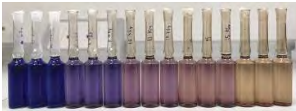
Radiochromic dosimeter extracted from a plant
