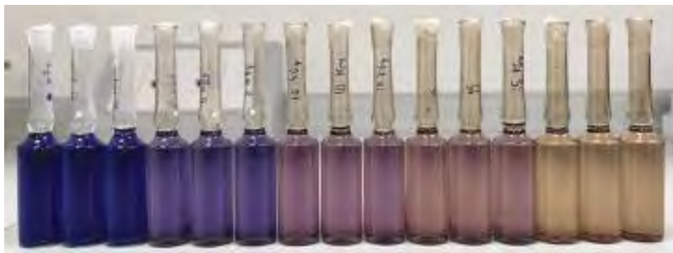
Radiochromic dosimeter extracted from a plant
