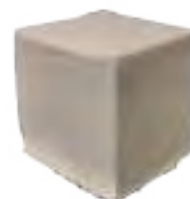
Heavy metal absorbent materials from natural rubber foam filled with gamma irradiated chitosan
